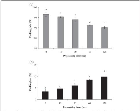
**Figure 2** The (a) cooking yield and (b) cooking loss of pre-cooked Pacific white shrimp. The shrimp were pre-cooked at 80°C for different times. Bars represent the standard deviation (n=3). Different letters on the bars indicate the significant differences (p < 0.05).
